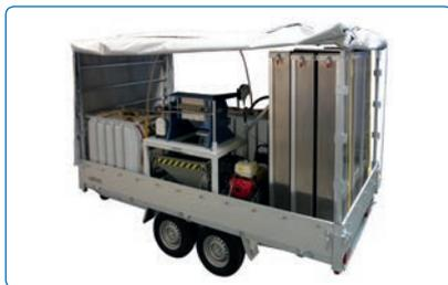
**Mobil waste water treatment system for resource recovery, as well as reduction of waste products**
