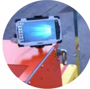
Integrated display which show a variety of different functions, from service message, blade rotation to tilt compensation and more.
